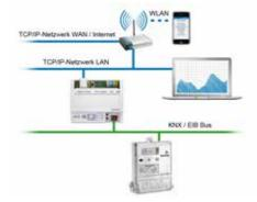
The integrated KNX data logger stores the data at 15 minute intervals over a period of one year. The data can be read out directly via the NK-FW network coupler using a standard Internet browser. By using FTP, you can also download the stored data from the KNX/EIB module for further processing, for example with MS Excel or Flash / Silverlight. The application program offers 15 data points for further processing in the KNX/EIB bus. The individual data can be transmitted cyclically to the KNX bus.
